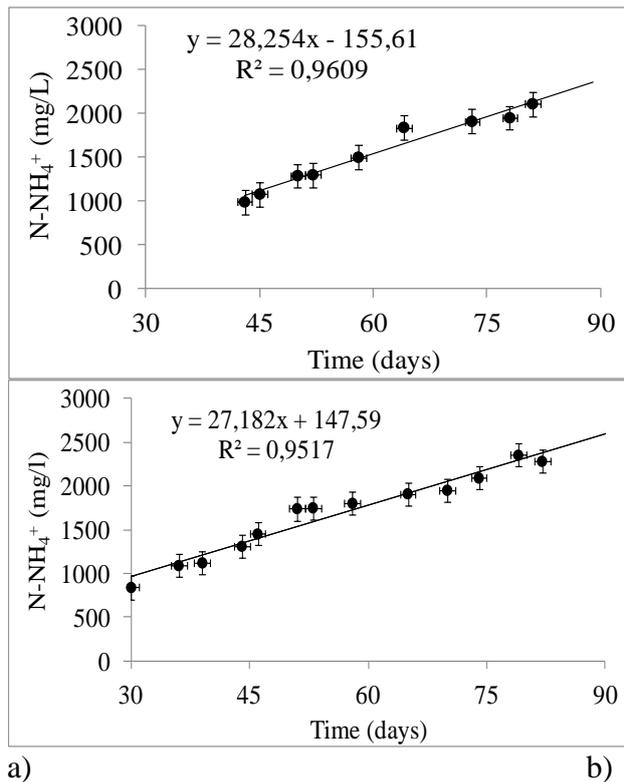
**Figure 27.** Ammonia accumulation rate a) in dark fermentation reactor; b) in anaerobic reactor.
