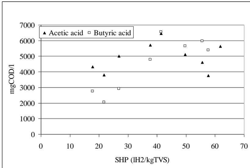
**Figure 22.** Relation between VFA and SHP during Run III.
