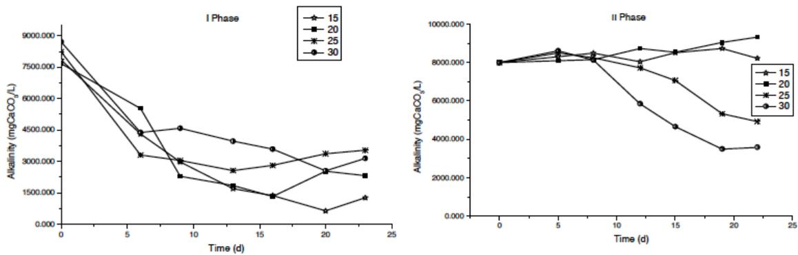
a) First phase alkalinity comparison, supernatant recirculation; b) second phase alkalinity comparison, supernatant recirculation.
