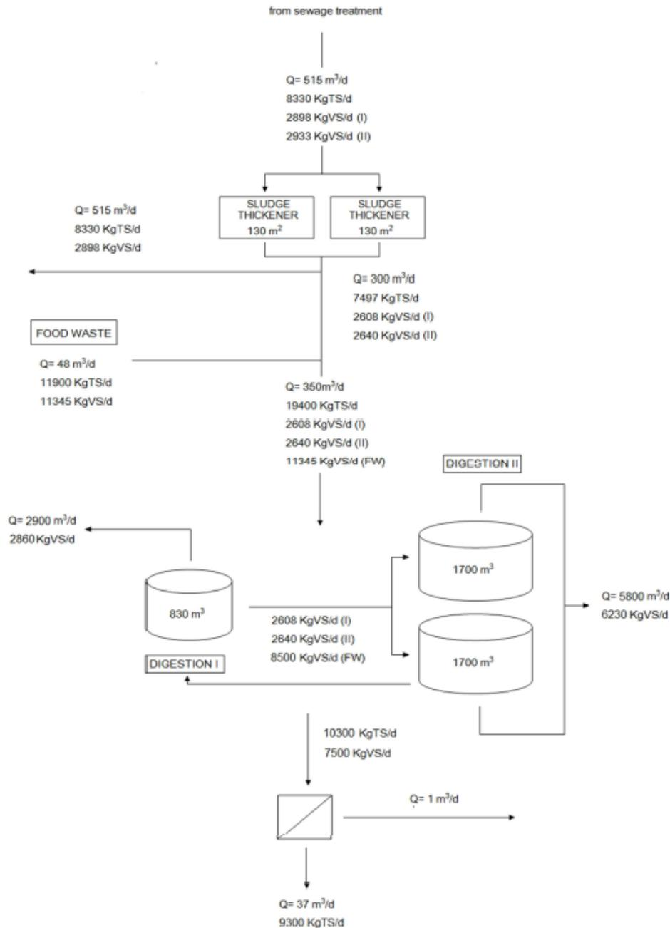
**Figure 31.** Scheme of the calculated mass flows for the sludge treatment line
