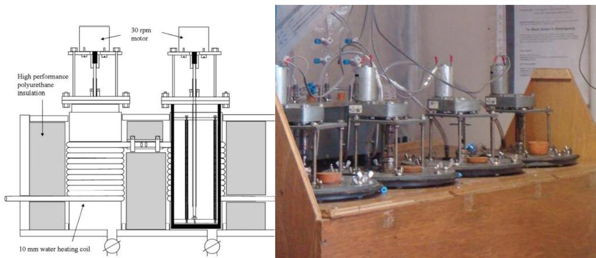
a) Cross-section diagram showing heating coils (left) and stirrer (right) (Banks et al., 2010)
