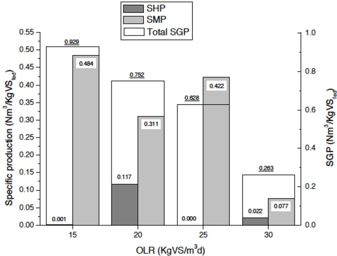
**Figure 18.** Specific Gas Productions for all the OLR tested with digestate recirculation
