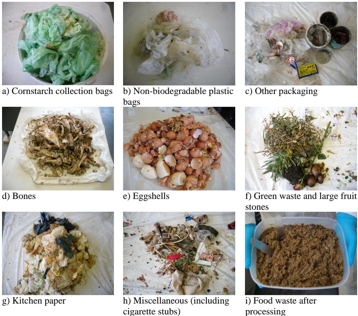
**Figure 3.** Cornstarch bags and contaminants found in food waste, materials removed to protect the grinder or laboratory-scale reactors, and food waste after grinding
