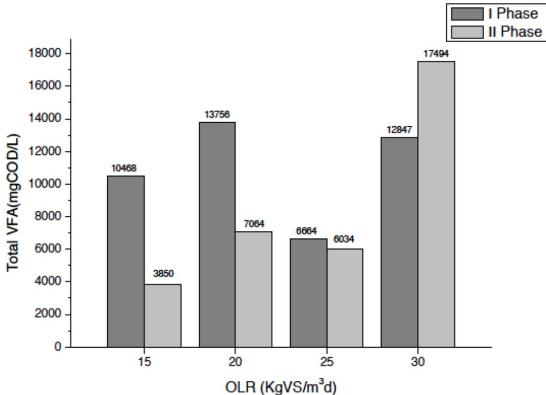
**Figure 19.** Total VFA for all the OLR tested with digestate recirculation
