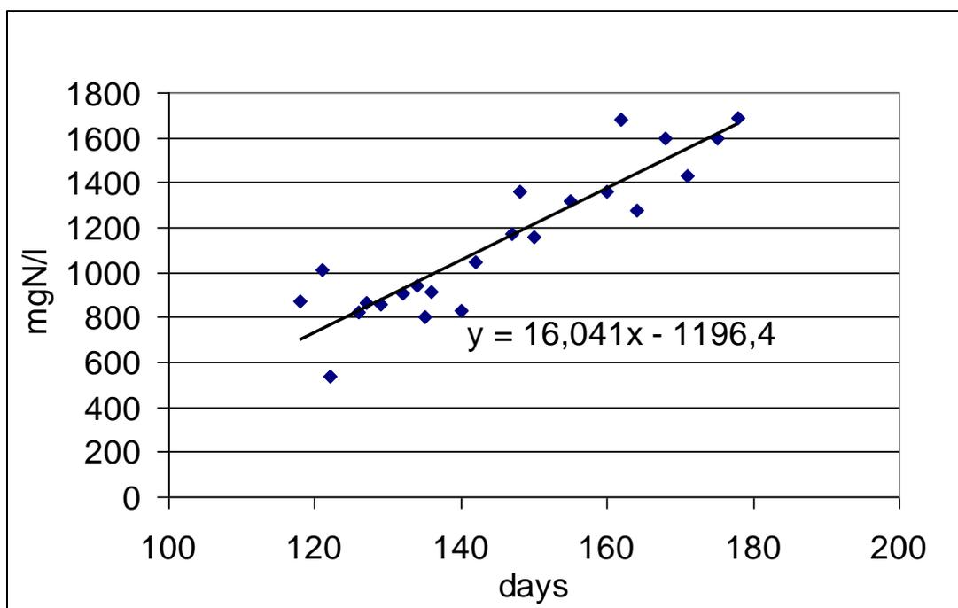
**Figure 25.** Rate of ammonia accumulation in second phase reactor Run III
