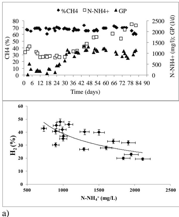
**Figure 28.** a) Effect of ammonia concentration in the anaerobic digestion reactor; b) Effect of ammonia on biohydrogen production in dark fermentation reactor.
