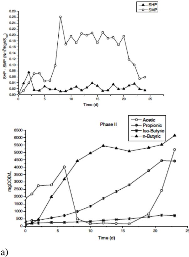
**Figure 17.** a) SHP and SMP trends with digestate recirculation, at  $\text{OLR } 30 \text{ kg VS m}^{-3} \text{ day}^{-1}$ ; b) acetic, propionic and butyric acid profile, second phase with digestate recirculation, at  $\text{OLR } 30 \text{ kg VS m}^{-3} \text{ day}^{-1}$
