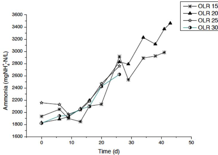
**Figure 20.** Ammonia accumulation during the second phase with digestate recirculation
