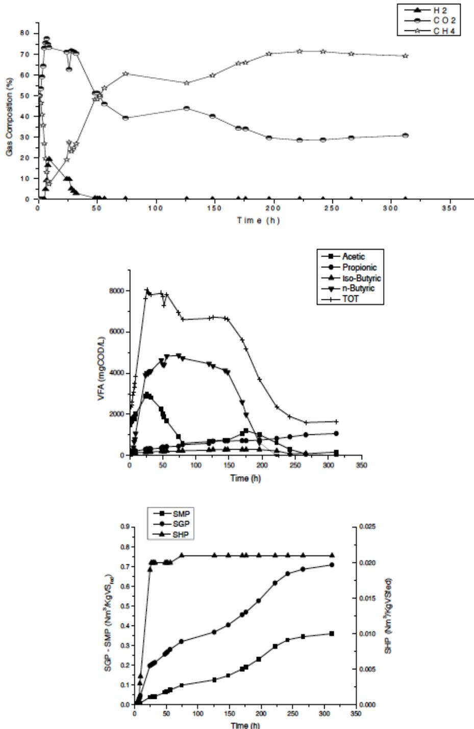
**Figure 9.** Gas composition, VFA and Specific Gas Production profiles for batch test at initial organic load  $20 \text{ kg VS m}^{-3}$
