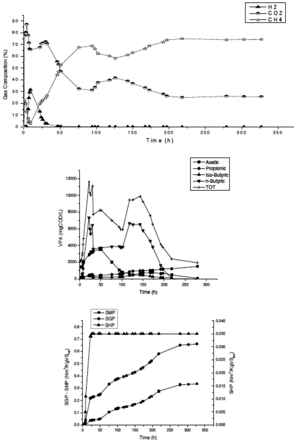
**Figure 10.** Gas composition, VFA and Specific Gas Production profiles for batch test at initial organic load  $25 \text{ kg VS m}^{-3}$
