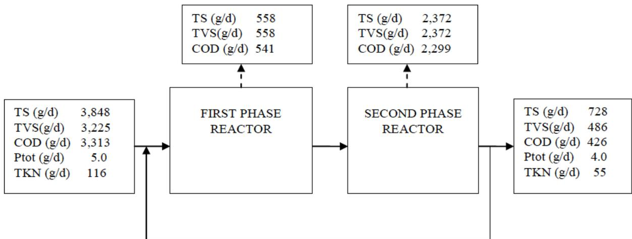
**Figure 24.** Mass balance of Run IIIa
